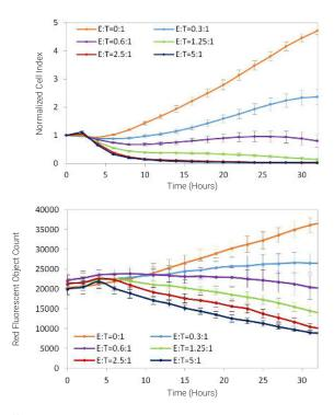
Effectors addition causes cancer cell death in a E:T ratio-dependent manner as shown by biosensor (top) and imaging (bottom) measurements. Red fluorescent object count indicates number of living target cells.
