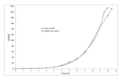
A high-cell density fed-batch cultivation of *E. coli* K12 in 3 L glass vessels and BioBLU 3f Single-Use Vessels, respectively, resulted in outstanding 200 OD<sub>600</sub> and highly similar growth curves—proving the excellent comparability of the vessel designs.
