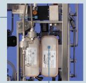
Optional glycol heat exchanger enables rapid cool-down; closedloop, eco-friendly design reduces need for single-pass cooling water
