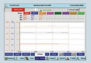
Trend graphs make it simple to track and export data on up to eight process variables over a six day span
