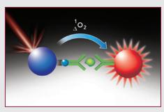
AlphaScreen® technology provides high signal:background ratios. The measurable energy transfer is emitted in the 520-620 nm.
