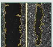
High throughput cell migration assays are enabled with AutoScratch Wound Making Tool, with timelapse imaging under environmental controls in Cytation 5.
