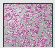
Use high contrast brightfield imaging for accurate label-free cell counting without the need for cell labeling dyes.
