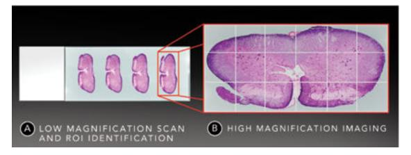
Cytation 7 and Gen5™ software facilitate ROI identification. Cytation 7 scans samples at low magnification before prompting the user to identify regions of interest to be imaged at high magnification. This greatly accelerates the process of imaging ROIs in batches of complex microscopic samples.
