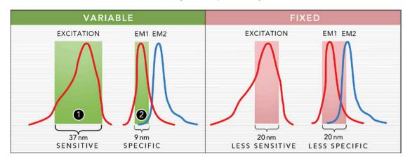
The plate reader optics of Cytation use a quad monochromator design with variable bandwidth. The bandwidth can be set anywhere between 9 and 50 nm in 1 nm increment. Large bandwidth settings (1) provide increased sensitivity and lower limits of detection. Small bandwidth settings (2) provide increased specificity when multiple signals are present, which reduces signal crosstalk and enhances assay performance.
