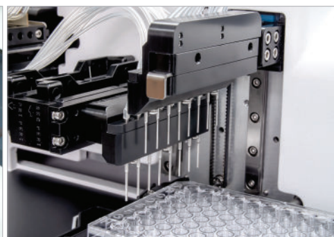
AMX module enables gentle media exchange for 3D cell cultures.
