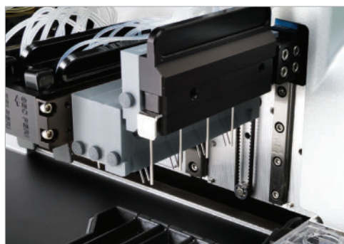
Wash 6- to 384-well plates with the wash module.
