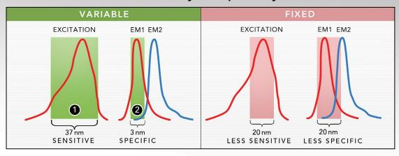
The Synergy Neo2 optics use a quad monochromator design, with variable bandwidth settings between 3 nm and 50 nm, in 1 nm increments. Large bandwidth settings (1) provide increased sensitivity and lower limits of detection. Small bandwidth settings (2) provide increased specificity when multiple signals are present, reducing signal crosstalk and enhancing assay performance.
