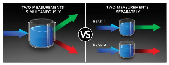
Two PMTs: Synergy Neo2 takes two measurements simultaneously. Other systems have to perform FP, FRET and TR-FRET measurements one at a time, which considerably lengthens the time to results.
