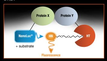
Bioluminescence resonance energy transfer (BRET) proximity assays enable detailed investigations of protein: protein interactions. BRET is easily detected with Synergy Neo2.
