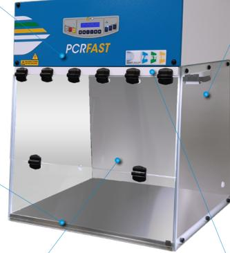
FRONT WINDOW AND SIDES PANELS MADE BY 6MM ANTI-UV SAFETY GLASS. A safety switch is in place to turn off UV when front glass is opened.
