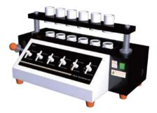
• F800-B use the same crucible system as F800, permitting samples to be dried and weighed between extractions if required.
