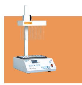
Each blowing needle can be controlled independently,the height of gas cavity is adjustable
